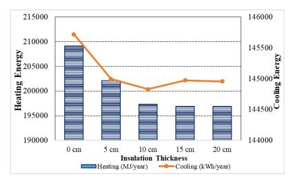
Figure 8. Variation of Energy requirements with insulation thickness
