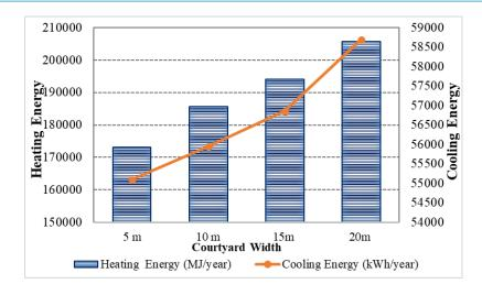
Figure 6. Effect of courtyard width on heating and cooling energy requirements
