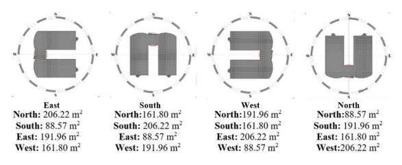
Figure 4. Window areas of different oriented building samples (Najib, 2019)
