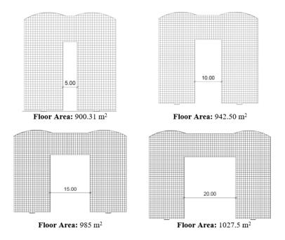
Figure 3. Building scenarios created with different courtyard widths (Najib, 2019)
